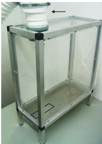
Fig. 1: BG Test Cage (front view). The air ventilation system is connected to the cage (black arrow). The arm is exposed at the test window in the metal floor sheet (black rectangle). The rear side is covered by gauze.
